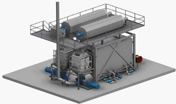
*Fish Draining and Weighing System - double*
