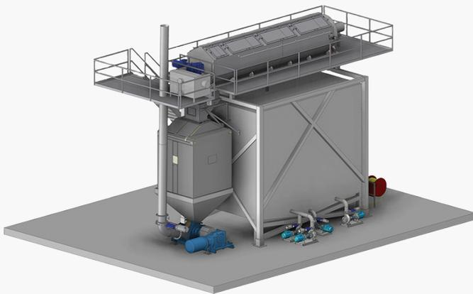
*Fish Draining and Weighing System - single*
