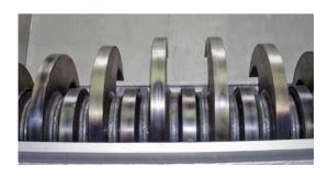
These large crushers are available in two configurations. The single-shaft unit can crush up to 15 tons/hour of individual frozen blocks, while the double-shaft unit is best for crushing whole pallets of frozen blocks, with an output of 50 tons/hour or more.
