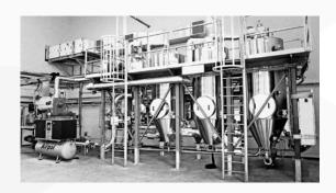
For continuous cooling of biosolids from thermal hydrolysis processes, for guaranteed compliance with temperature requirements in anaerobic digesters.
