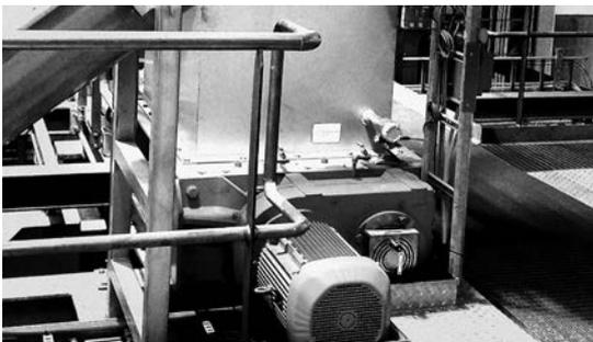
In many cases – usually because of there being many different types of packaging – it is easier and more cost-effective to crush such material first, rather than sending it directly to a depacker. The shredded material can then be passed through metal detection equipment, before passing on to the depacker setup.
