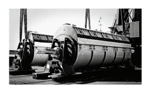
The Haarslev TST Disc Dryer is indirectly steam-heated and designed for high capacity, gentle drying and consistent product quality.
